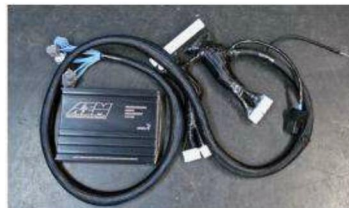
MP Tuning offers a custom extended wire harness for the S2000 AEM EMS to make installation a simple plug-and-play process.
